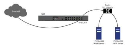
By enabling Routed Mode on the interface for the 172.16.6.0 network, NAT translations are automatically disabled for the interface, and all inbound and outbound traffic is routed to the WAN interface configured for the 10.50.26.0 network.
